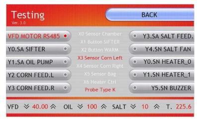
Fig. 7 Testing mode screen
