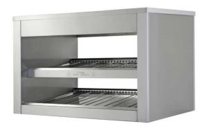
Tabletop open food display warmer with two warming shelves. Designed for demonstration and storage of pre-packed products. It is made of stainless steel. Components of the leading European manufacturers are used in the warmer's design. By implementing and combining glass ceramics heaters and heating cable, a steady temperature field is achieved across the surface of the shelf.
